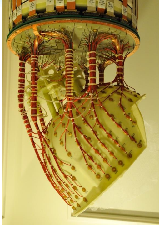
A basic SQUID Magnetometer. (Image: Adapted from DOI:10.13140/RG.2.2.17984.66564)
